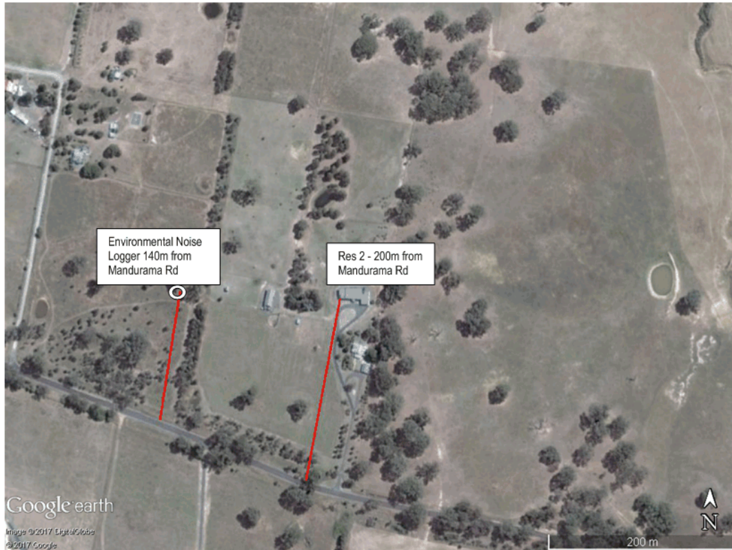
Map 2: Difference in distances from the road to the environmental logger and Res 2. Res 2 is further from the road and therefore closer to the external greyhounds than suggested.
